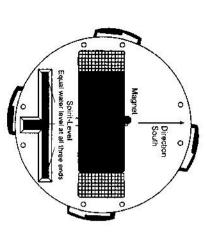
Alignment of Rain Sensor, Use of Spirit-Level and Position of Pickup Magnet
